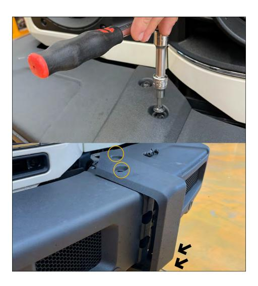
Remove the 4 screws on each of the right and left plastic holders, then remove the plastic holders.
