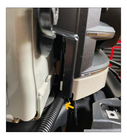
Guide the positive wire behind the vertically mounted cable.
