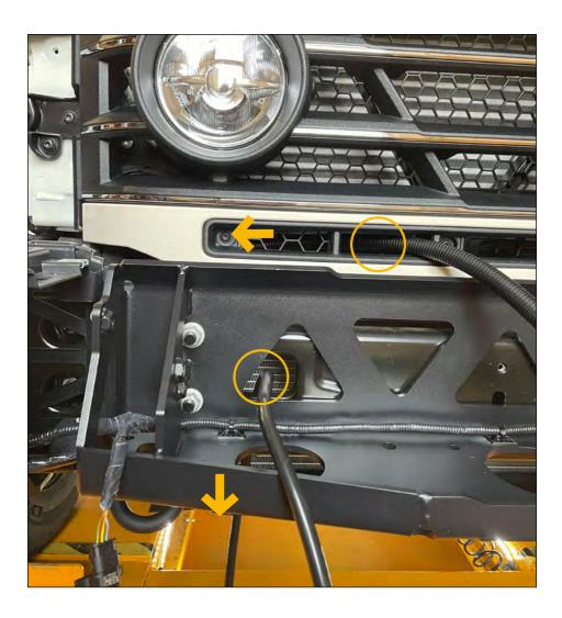
Thread the Warn Zeon 10 winch cables through the holes. (Cable routing instructions start on page 35)
