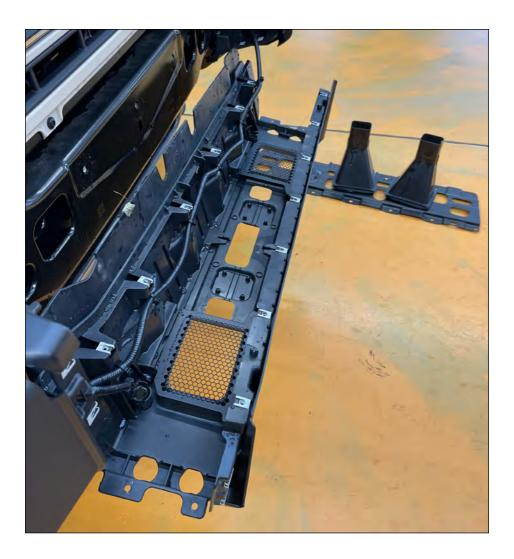
Remove the metal panel and the two underlying plastic air channels.
