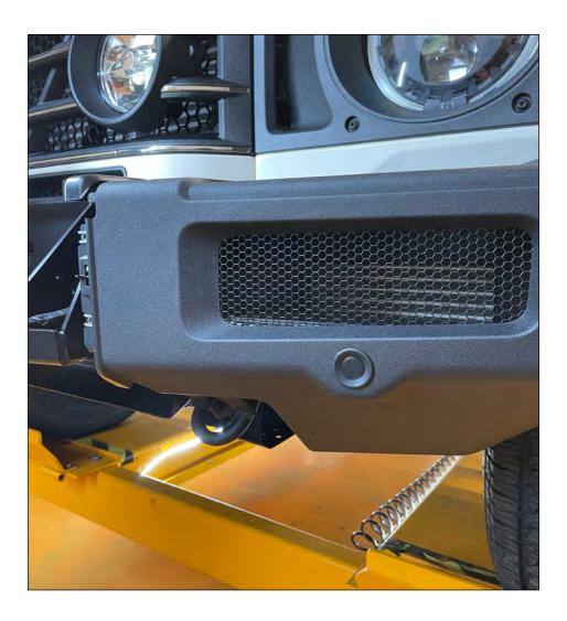
Reinsert the front left PDC sensor into its holder.
