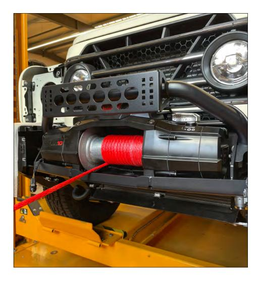
Plug the supplied remote control into the winch.
