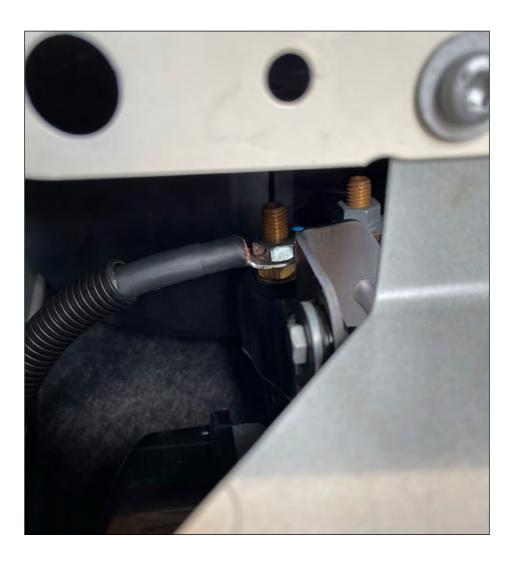
Attach the cable lug to the relay using an M10 nut.
