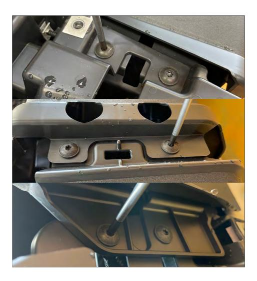
Remove 6 Torx screws per side (left and right).
