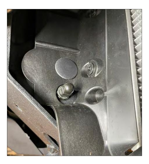
Unscrew the cap nut from the ground point.
