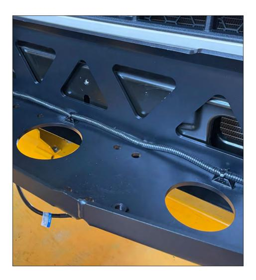
Fasten the cable harness using suitable mounting material.
