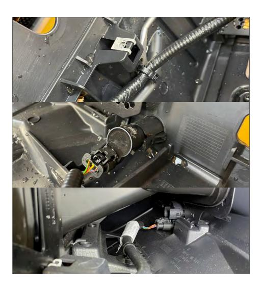
Disconnect the wiring harness with the PDC sensors from the center section and the front left of the bumper.
