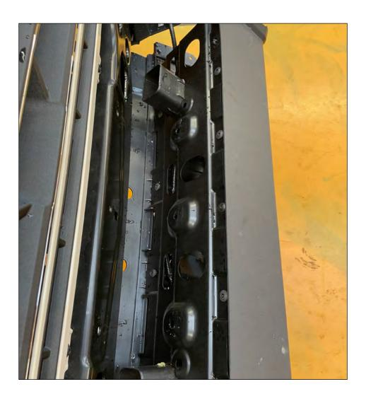
Remove 13 Torx screws from the rear side of the center part.
