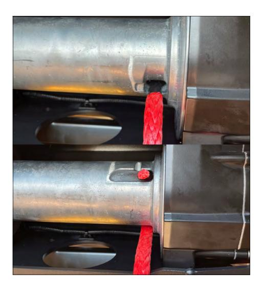
Pass the rope through the hole as shown.
