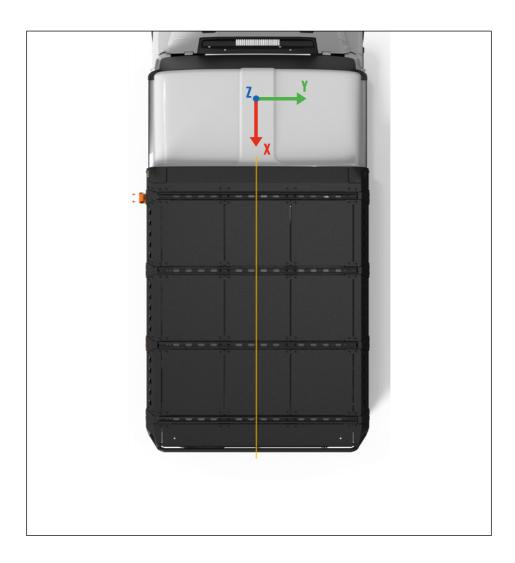
Place the LETECH roof rack on the roof so that the sealing lip at the front has about 5 mm clearance up to the roof phase.
