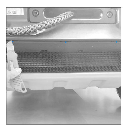
Remove the sprues in the bumper with a suitable tool.
