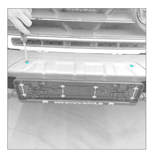
Loosen the two screws of the original winch cover and extend the cover from the bumper.
