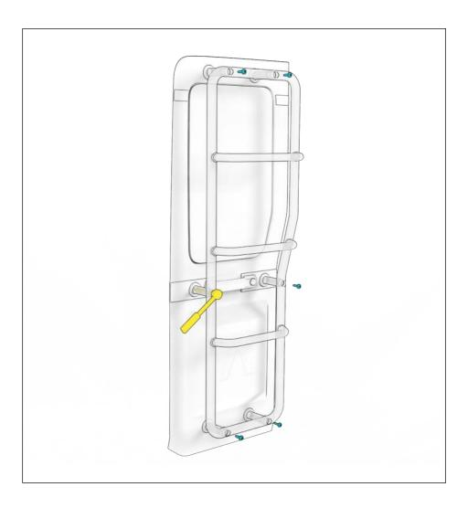
6x screw with TX 40 unscrew the key.
