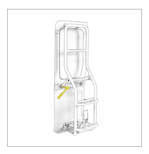
Provide the screws with screw lock "medium tight" and tighten with a 5 mm Allen key with 15 Nm.
