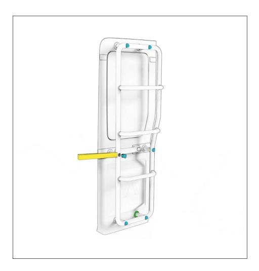
First dismantle the Grenadier rear ladder. Unscrew the sealing plug.
